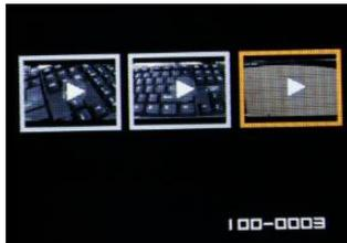
1. When DVR enters into recording mode, at this time press MODE twice, can go to the state of browsing 6 pictures 2. Press UP/DOWN to view pictures and videos. No press OK to enter into single mode, also
